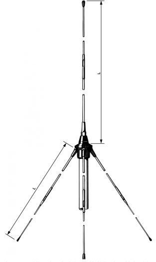
The radiator is measured from its free end to the bottom of the black insulator, while the radials are measured from their free ends to where they meet the GP-head.
